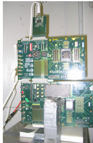
Fig. 3. Hardware Test Fixture for the Xilinx Virtex-5 Device
